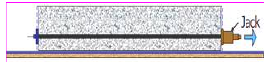
Placing of anchorage block & jack and applying tension to tendons
